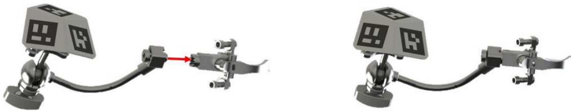
Figure 6: Assembling the Humeral Reference Rod to the Shoulder Humeral Ref
