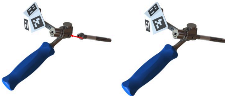
Figure 41: Assembling the Pin Inserter to the Adapter Handle
